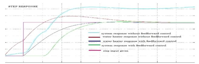
Fig 2. Step response of heating and humidifying sections of PEM fuel cell with and without feed-forward control
