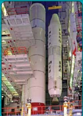
One of L40 Strap-ons being assembled to the core stage
