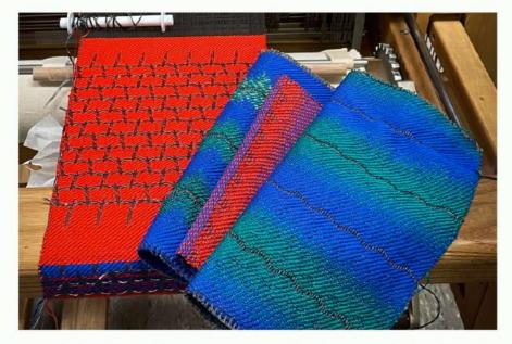
The team wanted to make a fabric "ear" that was soft, robust, comfortable, and could detect sound, based on the human auditory system. Their research led to two significant findings: Such a fabric would have to combine stiff, or "high-modulus," fibers to effectively transform sound waves into vibrations. In addition, the team would have to create a fiber that could bend with the fabric while also producing an electrical output.
