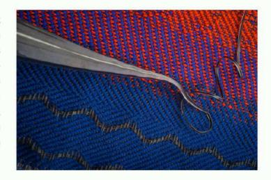
The fabric can detect sounds in a wide range of decibels, from a calm library to noisy traffic, and also detect the precise direction of quick sounds like handclaps. When woven into a shirt's lining, the fabric can detect a wearer's subtle heartbeat features. Audio, such as a recording of spoken words, can also be generated by the fibers and detected by another fabric.
