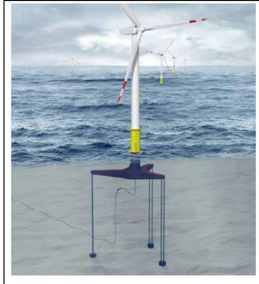
Fig. 3.6 PelaStar with tension-leg platform (source: www.ewea.org )
