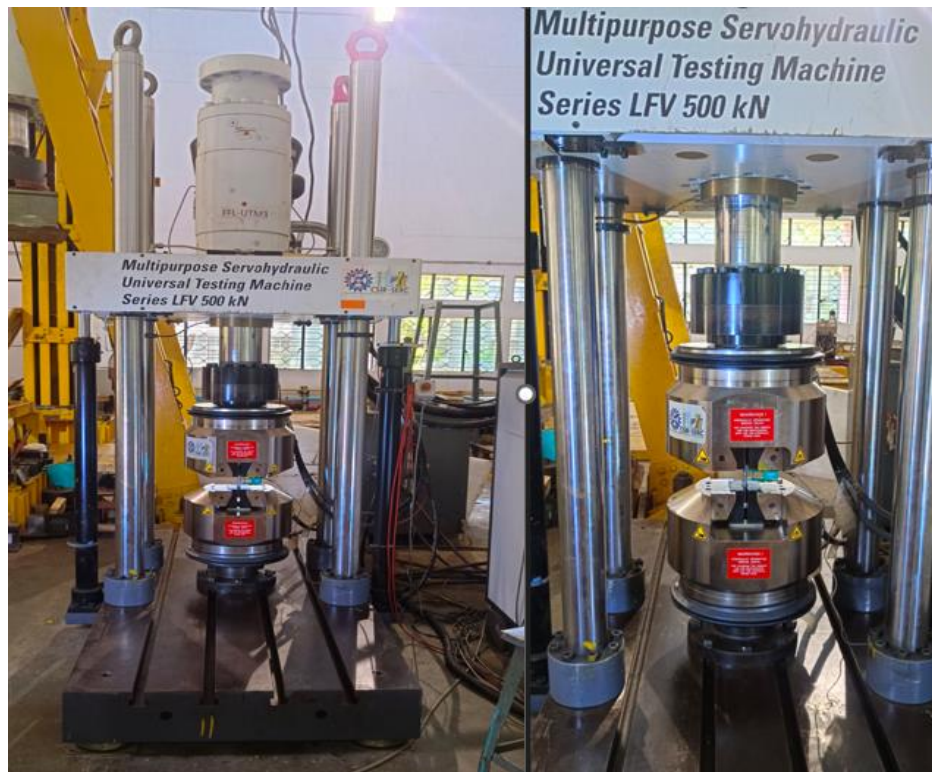
Fig. 5.6 Universal Testing Machine with tensile specimen included extensometer.
