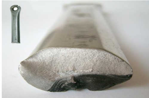
Fig. 1.9 Fracture of an aluminium crank arm. Dark area of striations: slow crack growth. Bright granular area: sudden fracture
