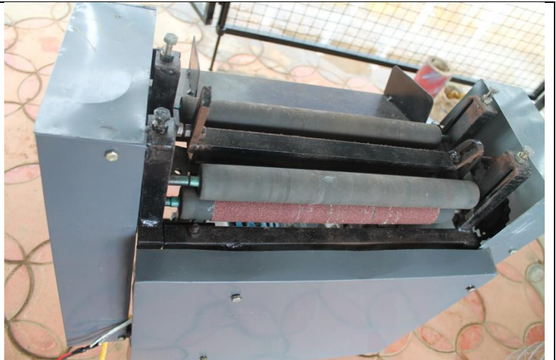
Figure 1 : Double rubber roller with spikers
