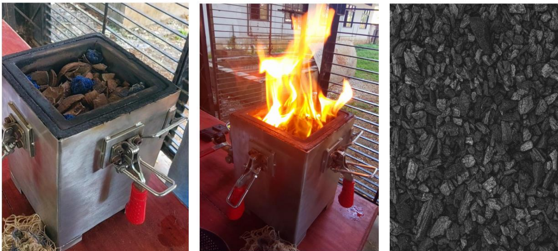
Fig 6.2 Preparation of biochar
