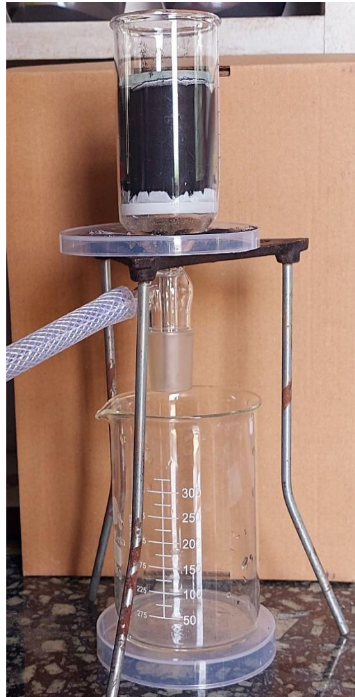
Fig. 9.8 Schematic diagram and conduction of column test
