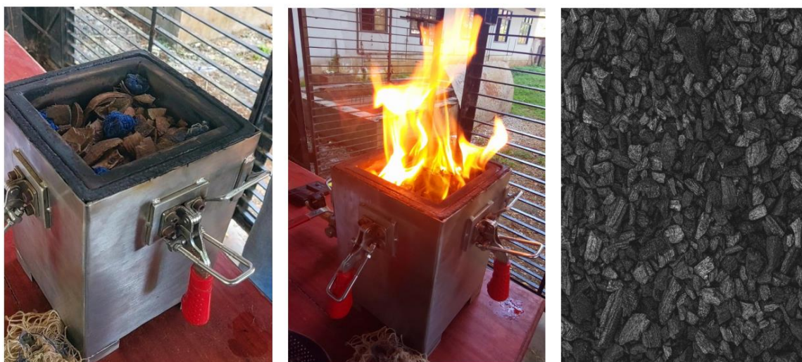
Fig 6.2 Preparation of biochar
